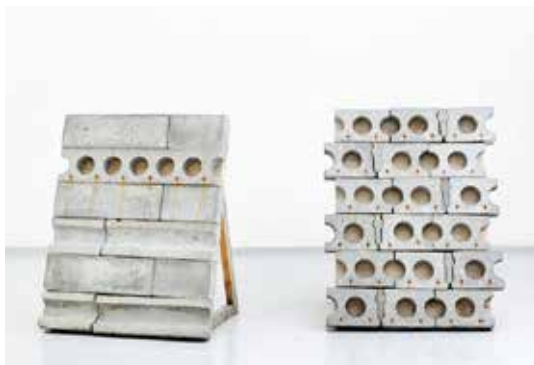
Figure 62 > Concrete bricks made from concrete slabs
