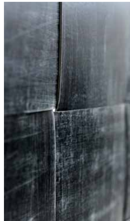
- Figure 55+56 Prototypes of Woven façade screens reusing rubber flooring (black) and vinyl (colored)
