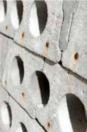
— Figure 5 Concrete bricks made from concrete slabs
