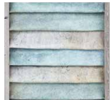
Fig 90-91 — Two versions of failed concept due to environmental reasons; vinyl flooring repurposed as façade panel.
